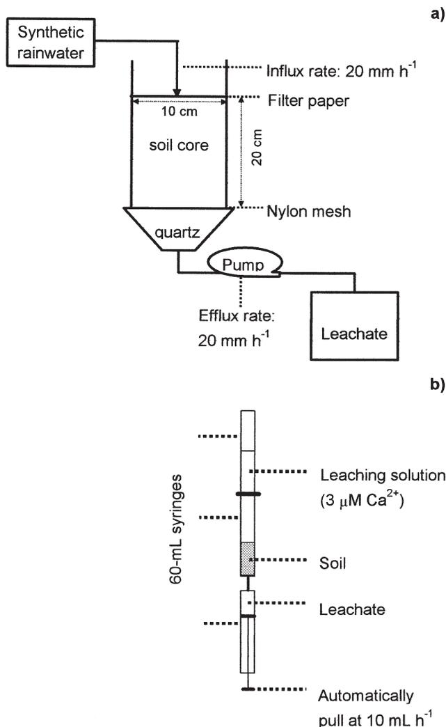
**Fig. 1. Schematic diagram of leaching apparatus used in (a) the intact soil core study and (b) the disturbed small soil column study.**
